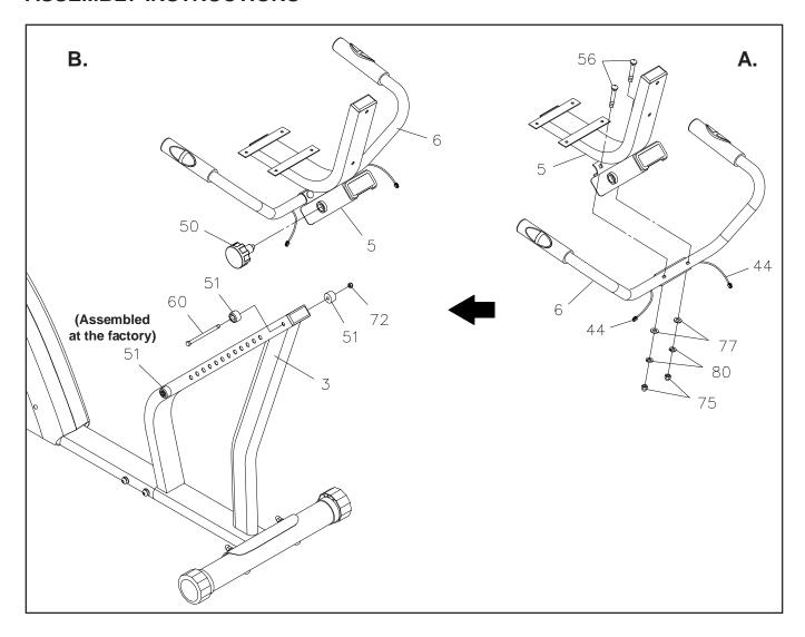
**NOTE:** Be careful not to damage the **PULSE SENSOR WIRES(44)** when attaching the **HANDRAIL(6)** and the **SEAT FRAME(5)**.
